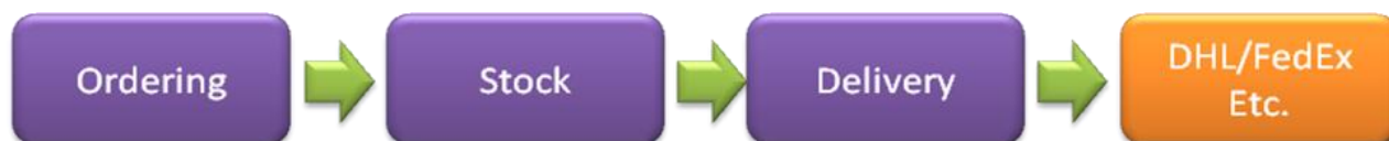
Figure 10.1 a vanilla ordering scenario. An ordering service sends the order to a stock service, which provisions the goods to a delivery service which is responsible to send the products to the customer
