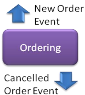
Figure 10.4 the Ordering service using the Inversion of Communications pattern. Now the service doesn't know/depend on other services directly. It is only aware of the business events of new order and cancelled order which are relevant to the business function that the service handled
